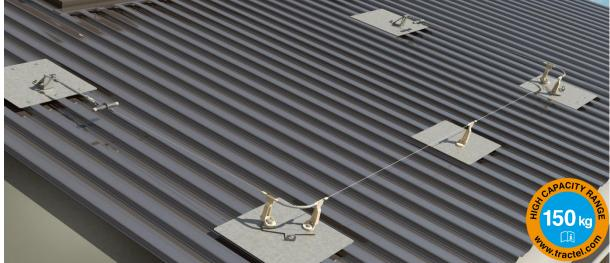
The Travflex<sup>™</sup> 2 single-cable system provides a smooth travel. It allows the slider to move freely over the intermediate anchors, minimizing wear and eliminating user assistance. The user's hands remain free to accomplish whatever task is required. It is designed to limit the forces transmitted to the structure in the event of a fall for installation on light structures such as steel deck roof.
