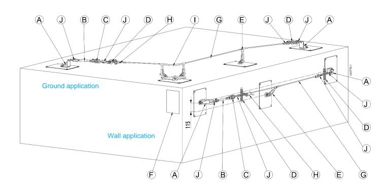
A. End anchorF. Information plateB. TensionerG. Wire ropeC. Tension indicatorH. Wedge socketD. INRS energyI. Corner kitabsorberJ. Quick link connectorE. Intermediate anchorF. Information plate
